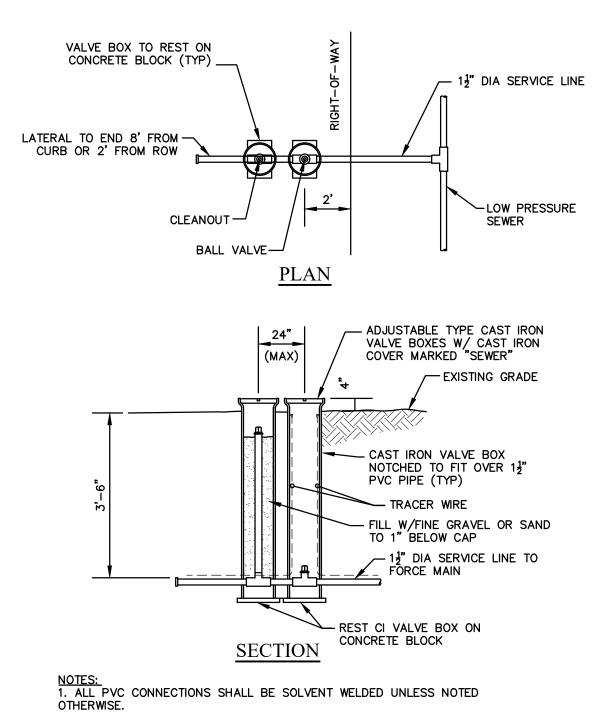
2. PROVIDE 6" OF AASHTO NO. 8 (OR PennDOT NO. 1B) STONE BELOW PIPE AND 12" ABOVE ENTIRE LENGTH OF PIPE.
