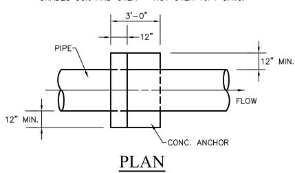
SPACING: GRADES 20% UP TO 35% - NOT OVER 36FT C.T.C. GRADES 35% UP TO 50% - NOT OVER 24FT C.T.C. GRADES 50% AND OVER - NOT OVER 16FT C.T.C.
